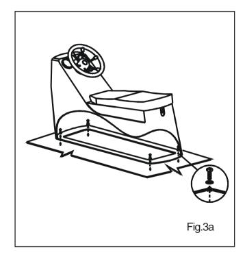
**ATTENTION !** To aviod the water penetration into the console and hull inner layers, please, tight all the hole free space with any water resistant filler.
